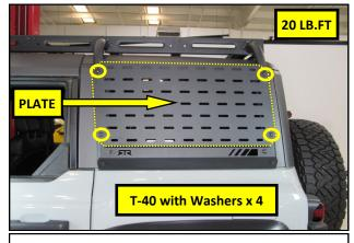
**2.** Set the Accessory Plate onto the vertical supports as shown and align the 4 sets of mounting holes. Secure the Plate to the uprights using the supplied M8 Button Head Bolts with Washers. Torque the Fasteners to 20 Lb.ft.
