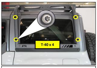
**1.** Using a T– 40 TORX<sup>®</sup> driver, remove the 4, Button Head Bolts in the RTR Rack vertical supports and set them aside. They will not be used with the RTR Accessory Plate.
