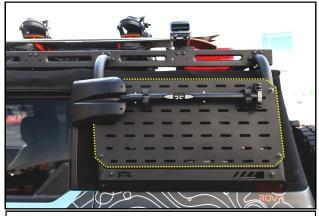
**3.** Mount accessories to the RTR Plate using the 1.5" MOLLE spacing in the Panel or by using the mounting components supplied with the tool or accessory. **NOTE:** some drilling or supplementary hardware may be needed to mount some accessories.
