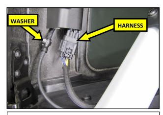
**4.** Disconnect the wiring harness and the washer fluid line.
