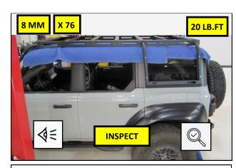
**53.** Inspect the Rack and verify that it is Square and Symmetrical –Adjust as needed. Using a T-40 TORX® driver, torque all M8 Fasteners to 20 Lb.ft. Remove the Blankets from the vehicle.
