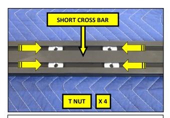
**24.** Locate the Short Crossbar and slide 4, T Nuts into the channels as shown.
