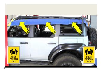
**41.** With the help of 3 assistants, and starting from the rear, carefully lift the Roof Rack up and onto the top of the vehicle.
