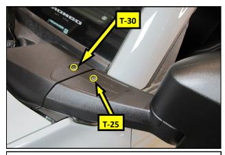
**18.** Using a T-25 and T-30 TORX® driver, remove the accessory screws in the mirror cover and mount.
