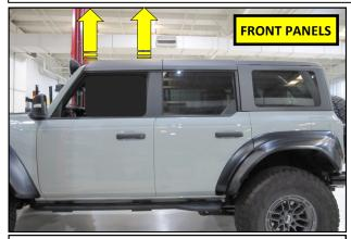
**1.** Remove the two front roof panels and set them aside.
