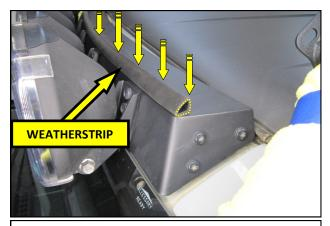
**38.** Peel the tape backer off of the Weatherstrip and apply it to the leading edge of the light bar as shown, with the forward facing edge swept rearward.
