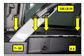
**12.** Using a T– 50 TORX® driver, reinstall the bolts removed in step **7**. Torque the bolts to 106 lb.in.
