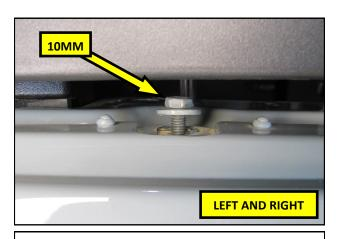
**8.** Loosen but do not fully remove the front bolt at the top of the rear fenders.
