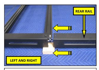
**30.** Slide the Rear (Short) Rails up to the No. 4 Cross Bar and onto the blocks.
