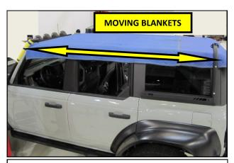
**40.** Drape a moving blanket or blankets across the entire length of the roof protect the vehicle.
