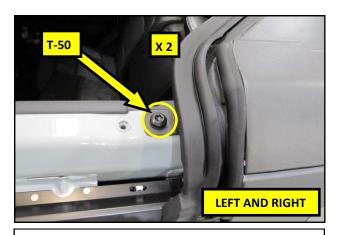
**3.** Using a T– 50 TORX® driver, remove the two bolts securing the rear of the top to the vehicle.
