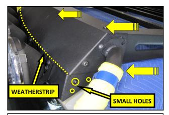
**42.** Slide the Rack forward, towards the light bar and over the weatherstrip. Align the small holes in the rack with the holes on the sides of the lightbar.
