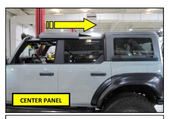
**15.** Using Slide the center panel rearward and secure it using the lock handles and latches.
