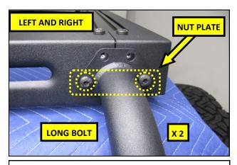
**46.** Secure the Rear Tube to the Rack using two M8 (Long) Bolts and the Nut Plate.
