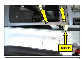
**6.** Raise the rear top and prop it up using blocks of wood.
