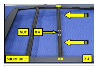
**28.** Slide the Cross Bars, one by one, between the Rails and align them with the holes in the Rails. Secure the Bars using the M8 (Short) hardware.
