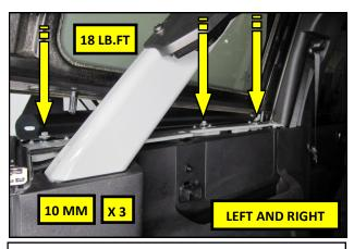
**10.** Tighten the fender bolts on both sides of the vehicle, from inside the cargo area. Torque the fender bolts to 18 Lb.ft.
