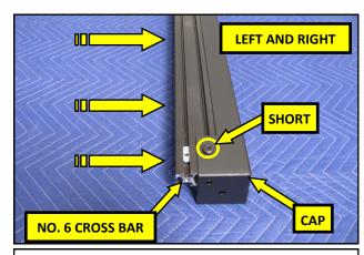
**33.** Slide the No. 6 Cross Bar with 4, T Nuts into the Rear Cap and secure it using 2, Short M8 Bolts.
