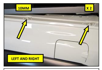
**7.** Using a 10 mm wrench, remove the two rear fender bolts on both sides of the vehicle.
