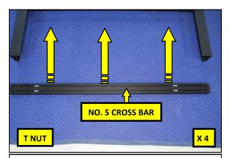
**32.** Slide the No.5 Cross Bar with T Nuts into the Rear Rail and secure it using four of the Short M8 Bolts.
