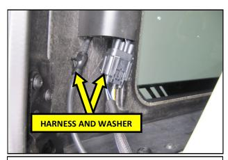
**13.** Reconnect the wiring harness and washer fluid line.
