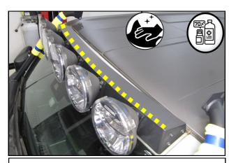
**37.** Clean the leading edge of the light bar using a mild solution of soapy water, followed by isopropyl alcohol.
