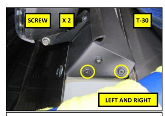
**39.** Using a T-30 TORX® driver, remove the two bottom screws on both sides of the light bar and set them aside.
