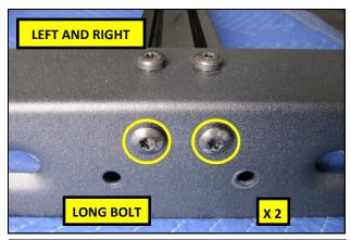
**50.** Secure the Cross Bars to the Rails using 2, M8 (Long) Bolts.
