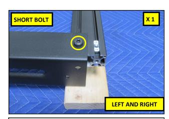
**29.** Place the ends of the Rails onto blocks of wood. Slide the No. 4 Cross Bar up to the first slot and secure it using a single M8 (Short) Bolt as shown.
