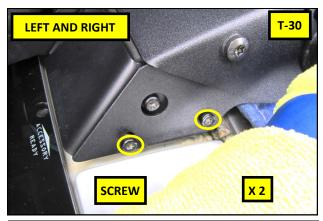
**44.** Secure the Rack to the light bar using the hardware removed in step **39**.
