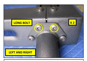
**47.** Thread in two M8, Long Bolts into the top two flange holes and into the Cross Bar.
