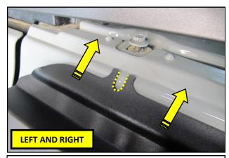
**9.** Slide the side specific Fender Mount between the fender and the top. When properly installed, the RTR logo will be on the leading edge of the Mount and the bolt from step **8** will be in the notch in the mount.
