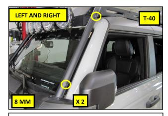
**54.** Install 2, M8 (Long) Bolts into the Front Tube.
