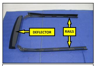
**21**. Lay the Left and Right Main Rails along with the Wind Deflector onto a padded work surface.
