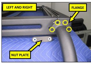
**45.** Align the holes in the Rear Tube flange with the holes in the side of the Rack. Place one of the RTR Nut plates inside the Rail, opposite of the flange.
