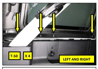
**5.** Using a T-50 TORX® driver, remove the 4 bolts securing the hard top on both sides of the vehicle.
