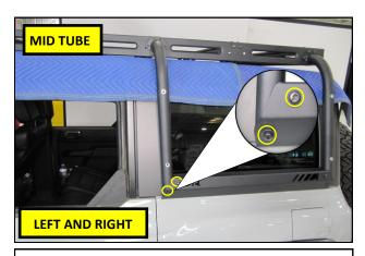
**48.** Using the supplied M8 Bolts with Washers, loosely install the Mid Tube onto the Fender Mounts, as shown.
