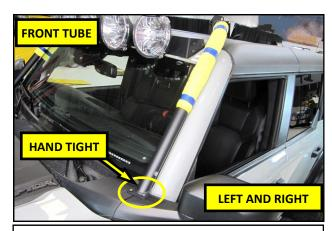
**20.** Using the OEM fasteners from step **18**, loosely install the Front Tubes onto the vehicle, as shown.
