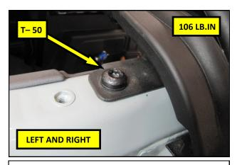
**14.** T- 50 TORX® driver, resecure the top to the vehicle using the hardware removed in step **3**. Torque the bolts to 106 lb.in.
