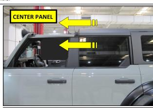
2. Detach and slide the center roof panel forward.
