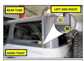
**17.** Using the supplied M8 Bolts with Washers, loosely install the Rear Tubes onto the Fender Mounts, as shown. **NOTE:** The Vertical Tubes are side and position specific. Location decals are on the mounting flanges of each Tube.
