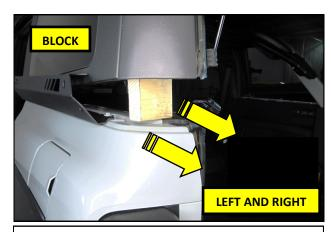
**11**. Remove the blocks and lower the top down onto the vehicle.
