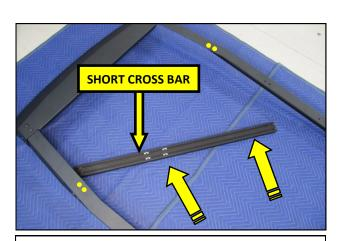
**25.** Slide the Short Cross Bar between the Rails and align it with the first set of holes in the Rails.
