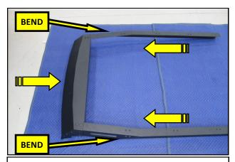
22. Slide the Rails and Deflector together as shown.
