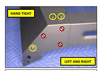
**23.** Secure the Deflector to the Rails using three of the supplied M8 x 25 (Long) Bolts. Leave these Bolts and all future Bolts hand tight until instructed to torque them.
