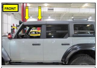
**16.** Reinstall the two front roof panels and secure them using the locking handles and latches.
