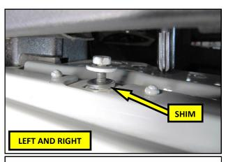
**RAPTOR MODELS ONLY:** Place the supplied shims on top of the upper fender bolt holes in all six locations.
