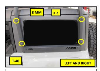
**55.** Install 2, M8 (Long) Bolts into the Mid and Rear Tubes. These additional fasteners and the unused Nut Plates are intended to allow for future accessories.
