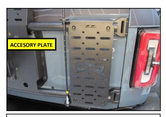
**7.** The RTR Antenna Mount can also be used in conjunction with the Accessory Plate, sold separately. Part Number: **14021.0011.14B**
