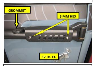
**4.** Using the supplied M8 button Head Bolts, install the Top Bracket as shown. When properly installed, the Top Bracket is on top of the tire carrier Hoop, with the ear and Grommet on the left. Torque the Bolts to 17 Lb.–Ft.
