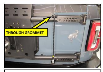
**6.** Mount the Antenna as shown, and in accordance with the manufacturers instructions. Use the supplied Cable Ties to secure the cable to the Bottom Bracket. Two sets of slots have been provided in the Bottom Bracket for this purpose.
