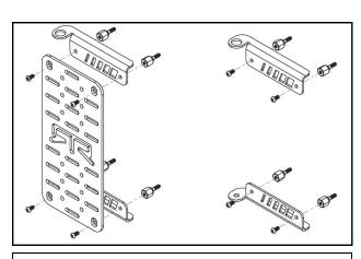
**9.** Alternative configurations using the RTR Accessory Adapter Kit, Part Number: **14025.0014.99.A.** on stock vehicles. **NOTE:** Alternative configurations will not use the M8 x 60 mm hardware included with the Antenna Mount.
