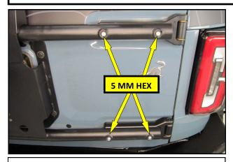
**1.** Using a 5mm Hex bit, remove the hinge bolts from the RTR Tire Carrier and set them aside.
