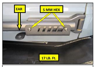
**5.** Using the supplied M8 button Head Bolts, install the Bottom Bracket as shown. When properly installed, the Bottom Bracket is on the bottom of the tire carrier Hoop, with the ear on the left. Torque the Bolts to 17 Lb.—Ft.
