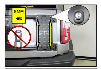
**3.** Mount the Accessory Plate onto the Tire Carrier using the supplied Button Head Cap Screws. RTR advises the use of Loctite® Threadlocker Blue 242, or equivalent, on all these fasteners. Torque the Screws to 17 lb.ft using a 5 MM hex bit, in like new condition.
