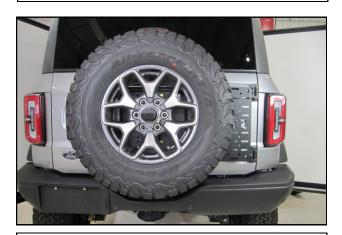
4. Reinstall the spare tire onto the carrier and torque the lug nuts to 41 Lb.-ft.
