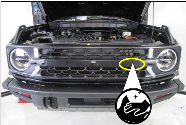
53. Clean the Badge recess on the Center Bar using isopropyl alcohol and a clean microfiber cloth.
