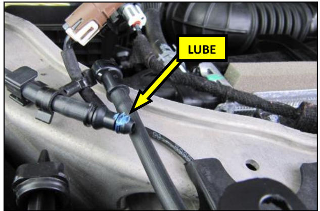
44. Apply a small dab of O-ring lube or silicone grease onto the O-ring on the male end of the washer hose.
