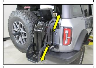
**45.** Open the Jerry Can Holder and place the fuel can inside of it as shown, with the handles facing forward and the filler neck facing rearward.
