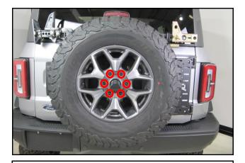
**37.** For vehicles equipped with the RTR Adjustable Spare Tire Carrier, remove the spare tire and set it aside
