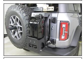
**46.** Close the Holder and position the can so that it has equal contact on all sides. Tighten the Spring Latch Nuts from step **18**.
