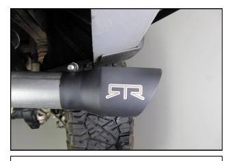
**4.** Retorque the adjuster Bolt following a thorough heat cycle.
