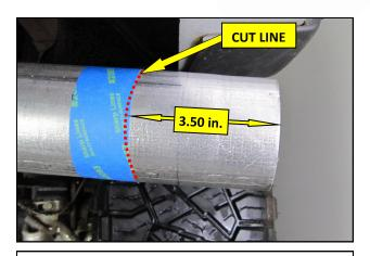
**1.** Slide the OEM tip off of the exhaust pipe, if so equipped. Using painters tape, mark a cut line 3.5 in. back from the edge of the OEM exhaust pipe.
