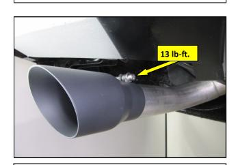
**3.** Slide the RTR Exhaust Tip onto the OEM pipe as shown, with the adjuster in the 12 O'clock position. Install the Bolt with the Washer into the adjuster and tighten the Fastener to 13 lb-ft.
