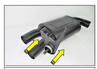
**8.** Reinstall the OEM exhaust hanger onto the RTR Muffler as shown, with the white half of the bushing facing rearward.
