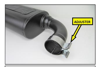
**9.** Slide the Clamp onto the Inlet Pipe as shown, with the adjuster furthest from the Muffler.
