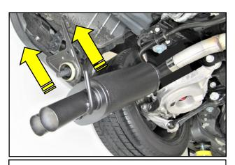
**10.** Slide the RTR Muffler Assembly onto the OEM pipe and rotate it upward, towards the vehicle.
