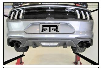
**15.** Align the second set of Tips with the first set and torque the Bolts. Retorque all of the Exhaust fasteners following a thorough heat cycle.
