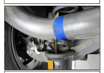
**3.** With the help of an assistant to brace the muffler, cut the OEM exhaust system using a Sawzall® or equivalent.
