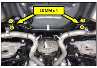
**5.** Using a 13 mm socket, remove the 4 bolts securing the sway bar to the vehicle and remove the bar from the vehicle.
