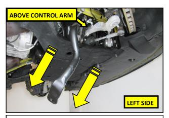
**18.** Raise the vehicle and working from the left side wheel opening, remove the sway bar, bushings and brackets.
