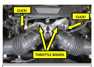
**31.** Reinstall the intake onto the throttle bodies and reconnect the vacuum lines.
