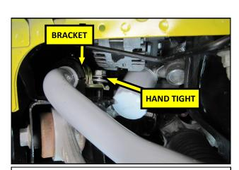
**22. LEFT SIDE-** Place the supplied Bracket over the Bushing and start the bolt removed in step **4** by hand.
