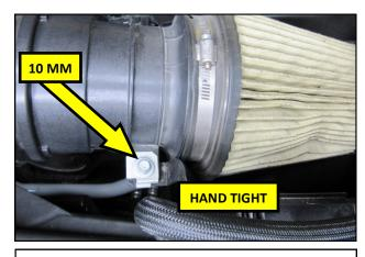
**33.** Secure the filter adapter to the airbox using a 10 mm socket the OEM hardware removed in step **9** .
