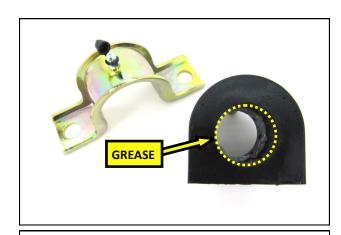
**20.** Apply a continuous bead the supplied Grease inside of each of the RTR Bushings.
