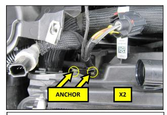
**15.** Using a panel clip removal tool, pry the wire harness anchors out of the fan shroud.
