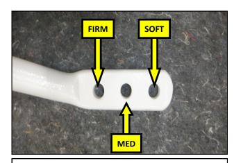
**TUNING**— The RTR Sway bar is adjustable and has 3 settings. RTR Recommends the Center position as a starting point.
