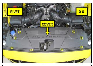
**36.** Reinstall the core support cover onto the vehicle using the plastic rivets from step **13**.
