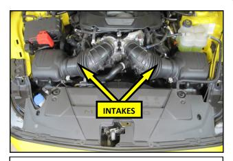
**5.** Lower the vehicle and raise the hood. The air intakes and air box lids will need to be removed.
