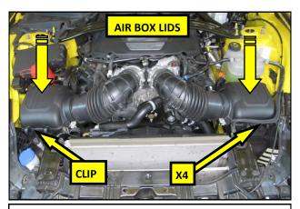
**35.** Reinstall the air box lids onto the intakes.
