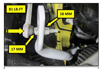
**26**. Slide the link studs into the Sway Bar and secure the links using the OEM nut removed in step **2**. Torque the nuts to 85 lb.ft.
