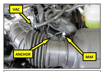
**6.** Disconnect the vacuum line quick connectors and separate the lines from the intake tubes. Disconnect the MAF sensor and pry the harness anchor out of the intake tube.
