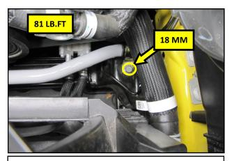
**23.** Secure the Left side bracket to the vehicle using the bolt removed in step **11**. Torque the bolt to 81 lb.ft.
