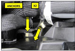
**29.** Install Reinsert the harness anchors into the fan shroud.
