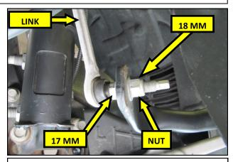
**2.** Using a 17 and 18 mm wrench, remove the sway bar nuts on both sides of the vehicle and set them aside.
