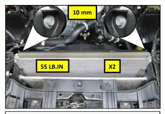
**28.** Secure the shroud to the radiator using the OEM hardware removed in step **16**. Torque the bolts to 55 Lb.in.
