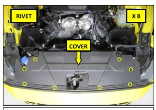
**13.** Remove the plastic rivets in the core support cover and remove the cover from the vehicle.
