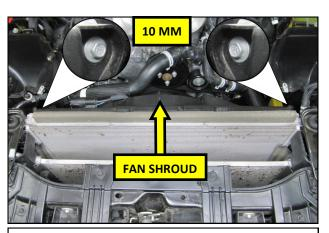
**16.** Using a 10 mm socket, remove the two flange bolts securing the fan to the radiator.
