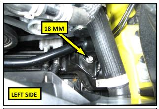
**11.** Using an 18 mm socket on a 24" extension, remove the forward bolt from the left side bracket.
