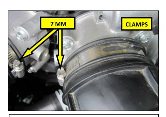
**8.** Using a 7 mm socket, loosen the throttle body clamps, but do not remove them.
