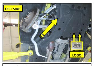
**19.** Working from the left side wheel opening, carefully slide the RTR Sway Bar into the vehicle. **NOTE:** when properly installed, the RTR logo will be facing upward.
