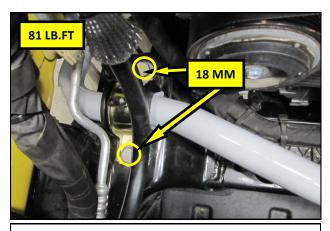
**24. RIGHT SIDE-** Secure the Right side bracket to the vehicle using the bolts removed In step **12.**Torque the bolts to 81 lb.ft.
