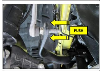
**3.** Slide the link studs out of the sway bar on both sides of the vehicle.
