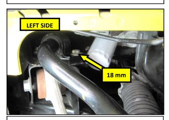
**4. NOTE:** The left rear, front bracket bolt is under the alternator and must be removed through the wheel opening. Using a 18 mm socket, remove the rear sway bar bracket bolt.
