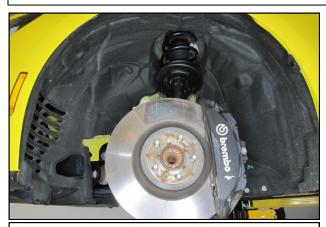
**1.** With the vehicle safely suspended on a hoist or jackstands, remove the front wheels and tires.
