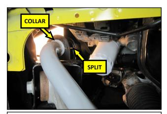
**21.** Spread the Bushings open and install them onto the Bar through the wheel openings. When properly installed, the bushings will be inboard of the shaft collars.
