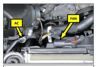
**30.** Reconnect the cooling fan and the AC pressure switch.
