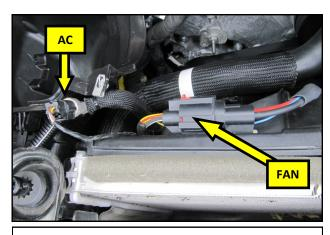
**14**. Disconnect the AC high pressure switch and the cooling fan.
