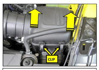
**7.** Unclip the airbox lid and remove the lids from the vehicle.
