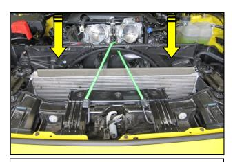
**27.** Remove the bungie cord and lower the fan back down into the vehicle. **NOTE**— Ensure that the tabs on the bottom of the shroud properly engage with the radiator and it secure.
