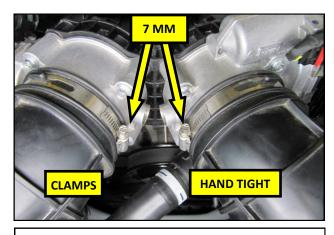
**32.** Using a 7mm socket, tighten the intake clamps.
