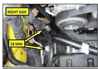
**12.** Using an 18 mm socket on a 24" extension, remove both bolts from the right side bracket.
