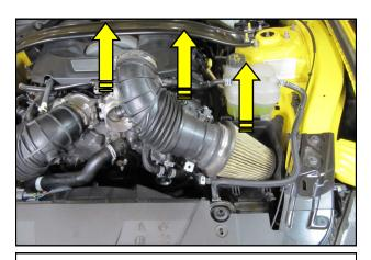
**10.** Remove the intake tubes and filters from the vehicle and set them aside.
