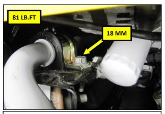
25. Torque the Left rear bolt from step 22 to 81 lb.ft.
