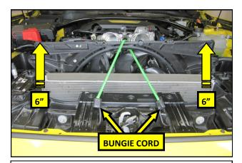
**17.** Raise the fan and shroud approximately six inches and secure it in the upright position using a bungle cord as shown.
