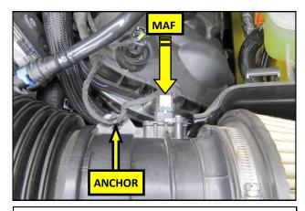
**34.** Reconnect the MAF and secure the harness by reinserting the anchor into the intake tube.
