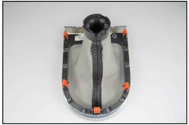
6. Place the boot and bezel assembly onto a padded work surface as shown.
