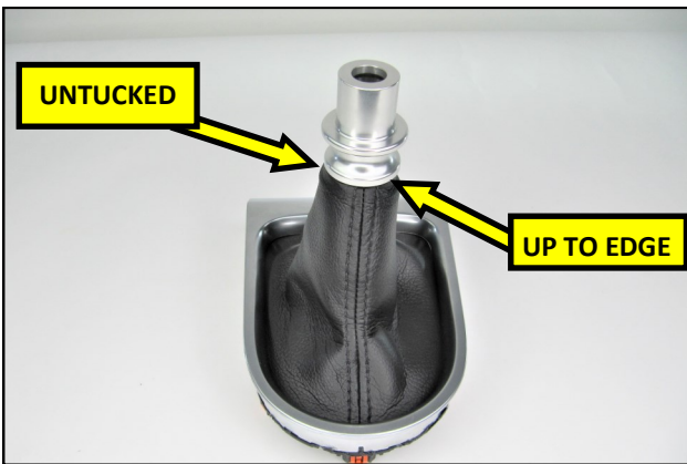
15. Driver's view of a properly installed RTR Lockout Collar.
