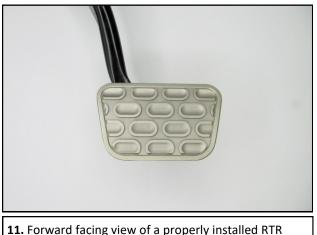
**11.** Forward facing view of a properly installed RTR Brake Pedal Cover.
