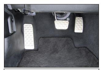
**CARE-** Clean the RTR Pedal Covers using a mild solution of soap and water. Avoid all caustic automotive cleaners with a PH of 12 or higher.
