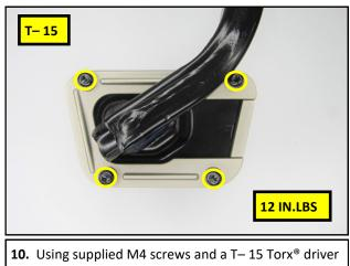
**10.** Using supplied M4 screws and a T– 15 Torx<sup>®</sup> driver secure the Retainer to the Cover. Torque the screws to 12 In. lbs.
