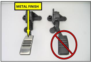
**NOTE:** The RTR Pedal kit is intended to be installed on vehicles equipped with the optional Accelerator Pedal with Metal Finish. New pedal assemblies can be special ordered from your local Ford Dealer if needed.
