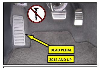
**1. Dead Pedal-Dead Pedal-2015 and newer models.** Locate and remove the dead pedal by prying it up and off of the floor of the vehicle. Inspect the 3 mounting slots in the floor for any retention clips that may have remained in the vehicle. Remove any clips that remain in the vehicle.
