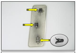
**12**. **Dead Pedal-2015 and newer models.** Push the 3 supplied Retention Clips onto the rectangular studs on Deal Pedal as shown.
