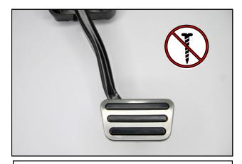
**6. Brake Pedal**– The OEM brake pedal cover has no mechanical fasteners securing it to the pad on the arm. It is non-bonded urethane with aluminum cladding.
