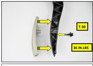
**4.** Using a T-30 Torx<sup>®</sup> driver, secure the RTR cover to the pedal arm using the supplied M6 Pan Head Screw and Washer. Torque the Screw to 36 in-lbs.
