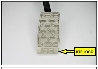
**5.** Forward facing view of a properly installed RTR Accelerator Pedal Cover.
