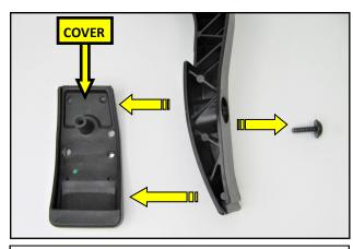
**3.** Remove the cover and screw from the pedal arm and set them aside. The OEM screw will not be reused with the RTR cover.
