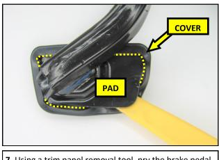
**7.** Using a trim panel removal tool, pry the brake pedal cover off of the pad and set it aside.
