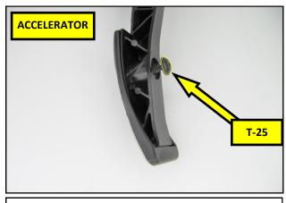
**2. Accelerator Pedal**– Using a T-25 Torx<sup>®</sup> driver, remove the screw from behind the pedal.
