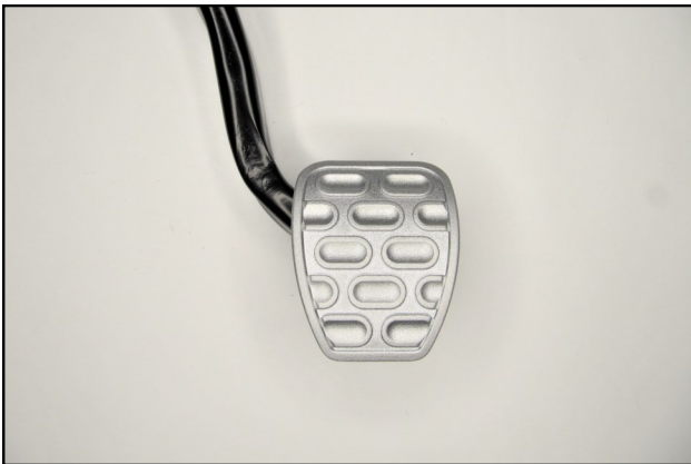
11. Forward facing view of a properly installed RTR Pedal Cover. Repeat steps 7-10 on the third pedal.
