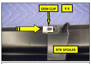
**19.** Reinstall the OEM speed clips from step **18**, onto the RTR Splitter as shown.
