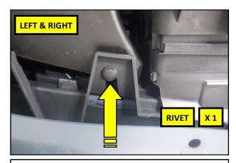
**29.** Reinstall the plastic rivet into the brake cooling duct inlet.
