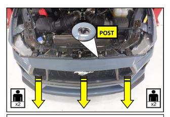
**14.** With the help of an assistant, lift the bumper cover up and over the core support posts and remove the cover from the vehicle. Place the cover, face down, onto a padded work surface.
