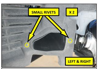
**3.** Remove the 2, small rivets in the brake cooling ducts, if so equipped.
