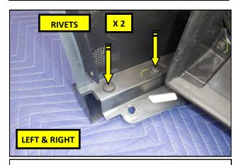
**21.** Secure ends of the Splitter to the bumper cover using the plastic rivets removed in step **16**.
