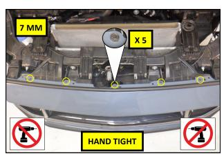
**24.** Using an 7 mm socket, reinstall the five OEM screws along the upper bumper cover. Tighten the screws by hand to avoid over tightening.
