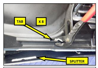
**17.** Using a pair of slip joint pliers, depress the splitter locking tabs one by one, from left to right, and remove the OEM splitter.
