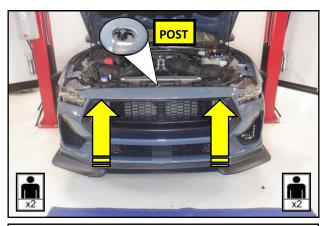
**23.** With the help of an assistant, lift the bumper cover back onto the vehicle and secure it onto the core support posts.
