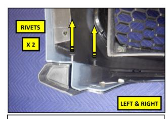
**16.** Remove the two plastic rivets from each end of the bumper cover as shown.
