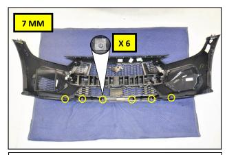
**15.** Locate and remove the six, chin splitter screws, using a 7mm socket.
