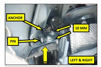
**27**. Lift the bumper cover up and press the fir tree anchor into the fender. Using a 10 mm socket, reinstall the two OEM bolts to secure the bumper to the fender. Repeat this step on the opposite side of the vehicle.
