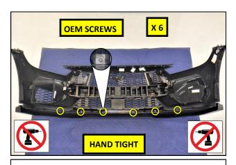
**20.** Mate the RTR Splitter to the bumper cover and engage the locking tabs, one by one, from left to right. Secure the Splitter using the screws removed in step **15.** Tighten the screws by hand to avoid over tightening.
