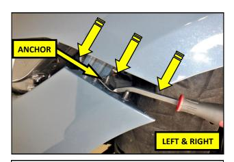
**10.** Using a panel clip removal tool, or equivalent, pry the fir tree anchors out of the fenders and separate the bumper cover from the fenders as shown.
