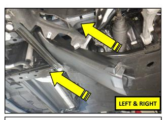
28. Reinstall the brake cooling ducts into the vehicle.
