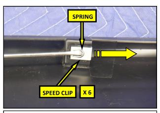
**18.** Using pocket screwdriver or equivalent, deflect the spring in the speed clip and remove the clip from the splitter. Remove the 5 remaining speed clips from the splitter.
