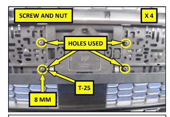
**8.** Using a T-25 TORX® driver and a 8 mm wrench, secure the Plate Mount to the Base Plate with the 5 mm Screws and Lock Nuts. Note the 4 holes used to mount the frame in the photo above.
