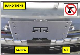
**6.** Using the Large Phillips Head Screws, secure the mount to the bumper cover, as shown. Tighten the screws until the Bumpers from step **4** come in contact with the bumper cover. Tighten by hand to avoid damaging the cover.
