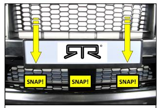
**10.** Close the Frame over the plate and snap the Frame shut. Verify the frame if fully closed and that the plate is secure within it.
