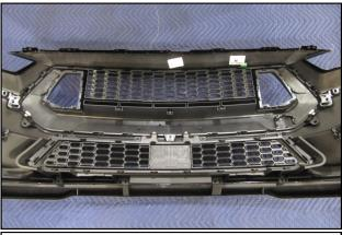
**1.** Place the bumper cover with the RTR Grille installed face down onto a padded work surface.
