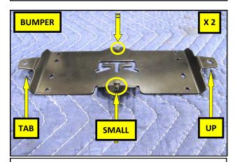
**4.** Place the Base Plate on a padded work surface as shown, with the mounting tabs raised. Carefully insert the Rubber Bumpers into the Mount, small side first.
