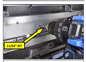
**3.** Using the Screw Bosses as guides, drill through the RTR Grille using an 11/64" bit.
