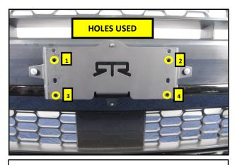
**7.** The Plate Frame is to be secured to the Base Plate using the holes indicated in the photo above.
