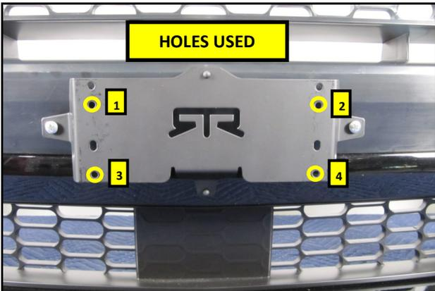
7. The Plate Frame is to be secured to the Base Plate using the holes indicated in the photo above.
