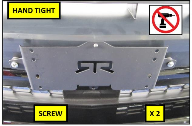
6. Using the Large Phillips Head Screws, secure the mount to the bumper cover, as shown. Tighten the screws until the Bumpers from step 4 come in contact with the bumper cover. Tighten by hand to avoid damaging the cover.
