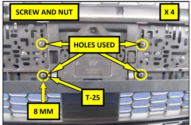
8. Using a T-25 TORX® driver and a 8 mm wrench, secure the Plate Mount to the Base Plate with the 5 mm Screws and Lock Nuts. Note the 4 holes used to mount the frame in the photo above.
