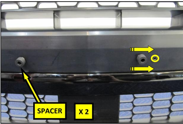
5. Place the rubber Spacers over the holes in the front of the bumper cover made in step 3 and align the holes.
