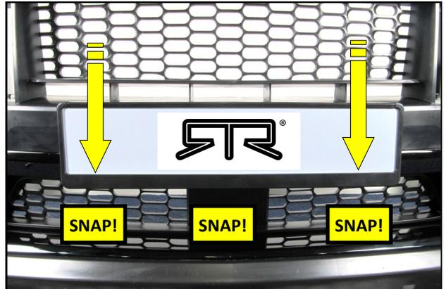
10. Close the Frame over the plate and snap the Frame shut. Verify the frame if fully closed and that the plate is secure within it.
