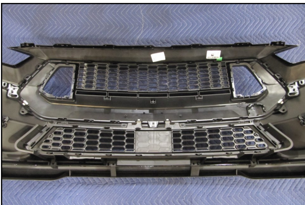
1. Place the bumper cover with the RTR Grille installed face down onto a padded work surface.
