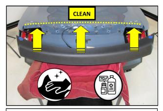
**31.** Clean the trunk lid, one last time, using isopropyl alcohol. Align the T bolts with the holes in the trunk lid and slide the RTR Spoiler onto the vehicle.
