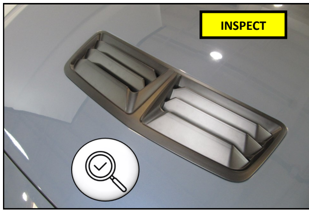
9. Inspect the installed position of the RTR Hood Vent and adjust if needed. The Install is now complete.
