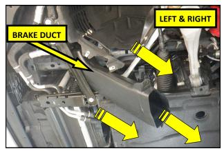
**5.** Remove the brake cooling ducts from the vehicle and set them aside.
