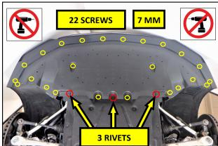
**30.** Lift the debris shield up and into the vehicle. Using a 7mm socket, reinstall the OEM screws and the plastic rivets. Tighten the screws by hand to avoid over tightening.
