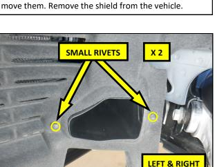
**3.** Remove the 2, small rivets in the brake cooling ducts, if so equipped.
