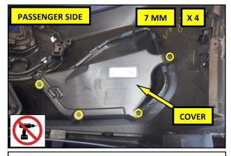
**21.** Using a 7 mm socket, remove the grille cover from the passenger side grille. Repeat steps **16-20** on the opposite side of the bumper cover and reinstall the cover using the OEM screws. Tighten the screws by hand to avoid over tightening.
