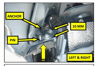
**27**. Lift the bumper cover up and press the fir tree anchor and guide pins into the fender. Using a 10 mm socket, reinstall the two OEM bolts to secure the bumper to the fender. Repeat this step on the opposite side of the vehicle.
