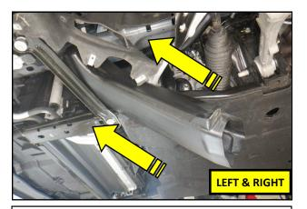
**28.** Reinstall the brake cooling ducts into the vehicle.
