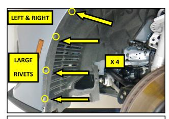
**32.** Unfold the fender liner and position it for reinstallation onto the bumper cover. Reinstall the 4, large plastic rivets into the front fender liners and cover.
