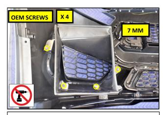
**20.** Using a 7 mm socket and the OEM screws removed in step 15, and reinstall the air duct as shown. Tighten the screws by hand to avoid over tightening.
