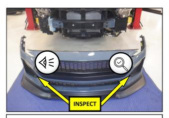
**22.** Inspect the installation from the front side of the bumper cover and confirm that all of the locking tabs are fully engaged and that there are no visible gaps.
