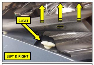
**13.** Carefully remove the weatherstrip foam from the cleat in the core support on both sides of the vehicle.
