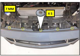
**12.** Using an 7 mm socket, remove the five screws along the upper bumper cover.
