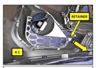
**16.** Depress the tab on the retainer clip and remove it from the bumper cover.
