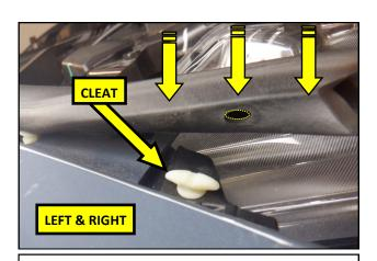
**34.** Carefully reattach the weatherstrip foam to the cleats on each side of the vehicle. Reinstall the wheels and tires to complete the installation.
