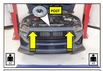
**23.** With the help of an assistant, lift the bumper cover back onto the vehicle and hang it onto the vehicle using the core support posts.
