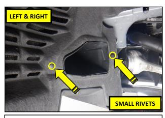
**31.** Reinstall the small plastic rivets into the cooling duct outlets.
