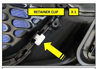
**19.** Reinstall the retainer clip from step **16** into the bumper cover.
