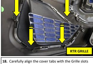
**18.** Carefully align the cover tabs with the Grille slots and install the RTR Corner Grille. Apply firm pressure around each tab until a distinct click can be heard, indicating full engagement.
