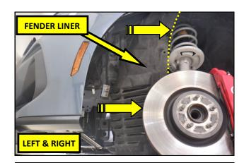
**8.** Gently fold the fender liners rearward, and behind the brake rotors as shown.
