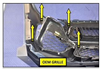
**17.** Depress the bumper cover tabs, one by one, and remove the OEM corner grille from the bumper cover.
