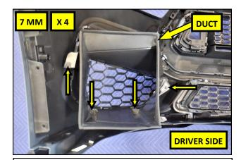
**15.** Using a 7 mm socket, remove the 4 screws securing the cooling duct to the corner grille. Remove the duct and set it aside.
