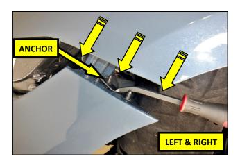
**10.** Using a panel clip removal tool, or equivalent, pry the fir tree anchors out of the fenders and separate the bumper cover from the fenders as shown.
