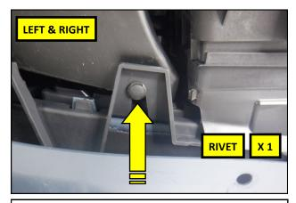
**29.** Reinstall the plastic rivet into the brake cooling duct inlet.
