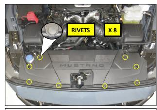
**33.** Reinstall the core support cover using the 8 OEM rivets removed in step **11**.
