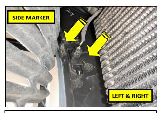
**25.** Reconnect the side marker lights on both sides of the vehicle.
