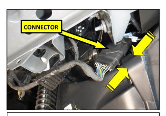
**26.** Reconnect the bumper wiring harness from step **7**.
