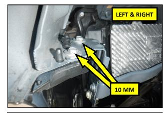
**9.** Using a 10 mm socket, remove the two bolts securing the bumper cover to fender. Repeat this step on the opposite side of the vehicle.
