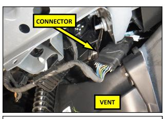
7. Locate and disconnect the bumper wiring harness.
