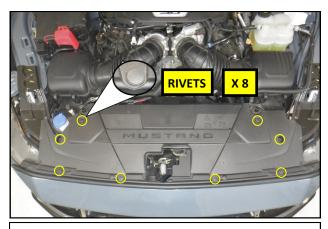
**11.** Remove the eight plastic rivets in the core support cover and remove the cover from the vehicle.
