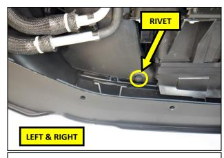
**4.** Remove the single plastic rivet in the cooling duct inlets.
