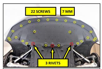
1. With the vehicle safely supported on a lift or jackstands, remove the front wheels and tires. Using a 7mm socket, remove the 22 screws in the debris shield. Pry the center post out of the 3 plastic rivets and remove them. Remove the shield from the vehicle
