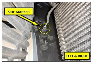
**6.** Locate and disconnect the side marker lights inside the bumper cover.
