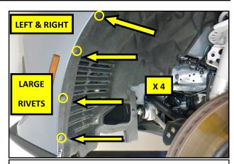
**2.** Remove the 4, large plastic rivets from both of the front fender liners. **NOTE:** This installation will reuse all of the OEM hardware. RTR Advises grouping the hardware by component to avoid confusion during reassembly.
