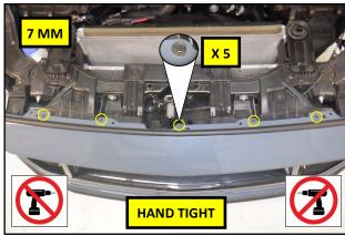
**24.** Using an 7 mm socket, reinstall the five OEM screws along the upper bumper cover. Tighten the screws by hand to avoid over tightening.
