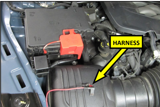
37. Remove the tape and rod from the RTR Harness and set it onto the air box cover at this time.
