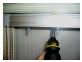
7. Insert stem replacement tool under the gear. Squeeze to release the louver stem.
