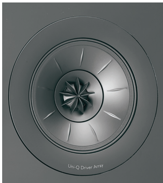
KEF's unique Uni-Q driver array, with central tweeter firing out through a shallow mid-range cone, dispersion controlled by Tangerine waveguides.
