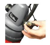
3. Screw the locking knob back into position, clockwise.
