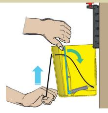
Once you feel it go over centre and start to release, slowly allow the setting cord to be drawn back into the trap, releasing the spring tension, and unsetting the trap.
