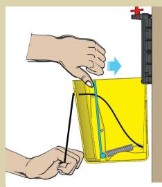
Gently push the back of the protruding bait bar forward, while keeping tension down on the setting cord.
