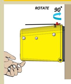
While supporting the top box with one hand, rotate the red button 90 degrees to unlock it.
