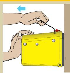
With the palm of one hand pushing against the top surface, use the other to pull the resetting cord firmly toward you until you feel the trap is set.
