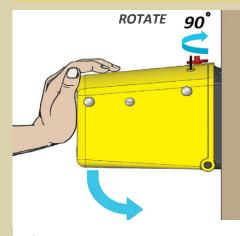
Support the top box with one hand and rotate the red button 90 degrees to unlock it. With the top box now free to pivot, guide it downward until it comes to rest on the tree or post.
