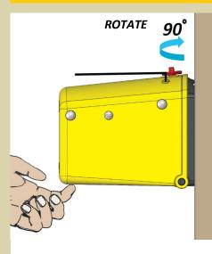
While supporting the top box with one hand, rotate the red button 90 degrees to unlock it.
