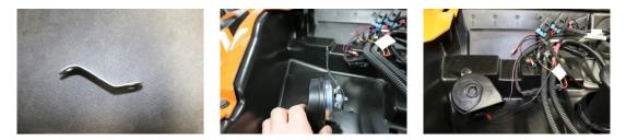
Connect the violet wire to one of the horn terminals and the black wire provided to the other terminal, run the black wire over to Buss Bar and attach to ground. If the car has not been upgraded with the Buss Bar Power Up Kit or Winch Kit, then the black wire will need to be grounded to the buss bar mounting screws
