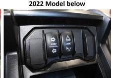
**Dielectric Grease** - Just like the OEM uses on their switches, we recommend using Dielectric Grease on all switch terminals, this keeps the water out, thereby reducing corrosion and helps increase reliability! Open the grease and put on the switch terminals and the connector terminals on both the Turn and Horn switches, the more the better.
