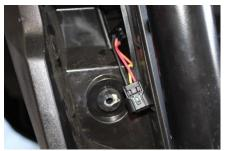
5. Run the two connectors with the green wire through the rear channel, above the heat shield to the passenger side, secure harness with provided cable ties. Plug in line with right taillight and reinstall light.
