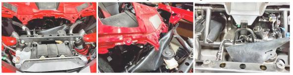
Remove Center Console Plastics and Rear Box Cover to run rear harness.
