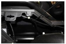
6. Plug the extension cable into the rear harness, run the 4-pin connector up behind the battery, into the center down behind the airbox, follow the factory wire harness to the center console, all the way up to the Control Module and Plug-in. Keep it away from any **HOT or MOVING** parts. Using the provided Cable Ties secure it to the main OEM wire harness
