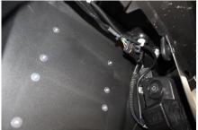
7. Install Front LED Turn Lights, the front LED Turn Indicators can be mounted with the rubber grommet or without. If the grommet is **not** being used drill 5/8" holes. If the grommet is being used drill ¾" holes. Remove and install the rubber grommet from the LED into the hole if being used. Insert LED into the hole with the Top marking up. NOTE: the TOP marking is on the front of the LED lens.
