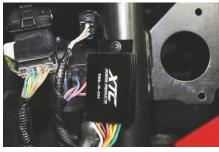
3. Unroll the long extension harness and the short Rear Harness. Remove both taillights by pulling out on the bottom and then pull back. Remove the rear box cover as shown by arrow.
