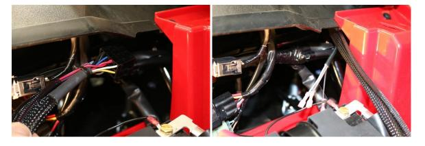
**CAUTION:** Verify there is proper clearance behind dash for the switch before cutting!
