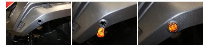
Insert the grommet into the hole, take the wires from the LED and insert into grommet, the LED has a TOP mark on it, insert it into the grommet with the TOP up.
