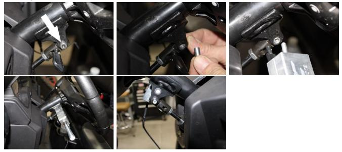
Install the Horn/Hazard Switch. On Pre 2021 models, use a new sharp razor, cut switch rectangles out. Do not over cut, try inserting switch and trim as necessary. It helps to rock the razor to cut. On newer models, remove one switch plug. Run the Horn wire connector through the rectangle switch cutout and use included grease on terminals, connect to switch and slide switch into dash.
