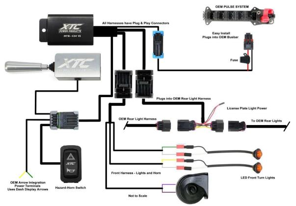
1. Remove the Hood and part of the dash cover. Mount the Control Module using the self-tapping screw provided.
