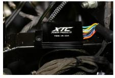
3. Plug Rear Harness into OEM Ride Command 8 pin Connector - Unplug the wire harness at the rear left side and connect our harness inline. (Note: There is a Red and Black power wire provided for an optional license plate light). Reach into the rear and unplug the center brake light and plug the harnesses 4 pin into it. If your RZR does not have a third brake light, one can be added or just ZIP tie the harness under the rear.
