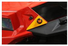
Run the short front harness through rubber grommet to the control module and plug in. Run the green wire to the right (passenger) side and connect the green wire to the black and the white to white. Run the yellow wire harness to the left (drivers) side, yellow wire attaches to black wire and the white wire goes to white. **NOTE: Black wire is positive and will not work if reversed. White is ground. Secure the Harness using the provided cable ties.**
