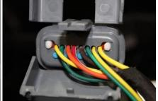
Close Cover – Run ATS wires alongside the OEM harness and snap shut, re-install plastic locking cover and plug back in.
