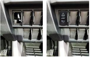
Run Switch Harness–Plug the Switch Harness into the Control Module, run Horn/Hazard connector through the rectangle switch cutout and use included grease on switch terminals then connect Switch and slide into dash. **NOTE:** The switch cut
