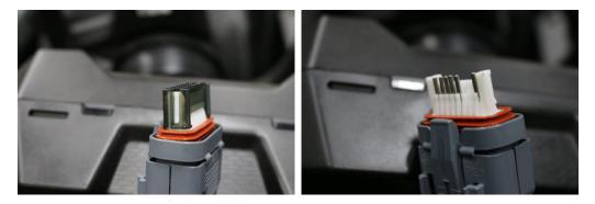
10. Remove Plugs – Using a pair of needle nose pliers remove the plugs from wire port 6 and 7, insert green wire terminal into 6 and yellow wire terminal into port 7.
