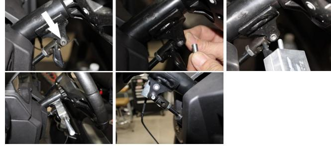
7. Install the Horn/Hazard Switch. Remove 1 of the switch plugs.
