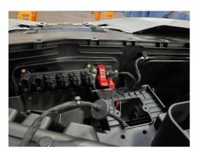
2. Mount the Control Module using the screw provided. Mount just to the side of one of the holes for Relays
