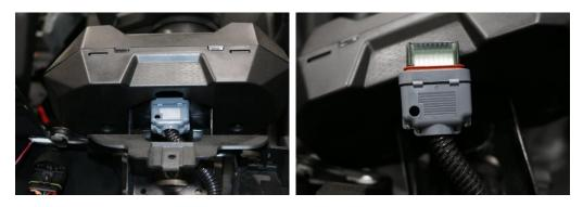
9. Remove Connector Lock – Using a small screwdriver push in on both sides at the white connector shown below and slide lock off
