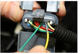
11. Close Cover – Run ATS wires alongside the OEM harness and snap shut, re-install plastic locking cover and plug back in.
