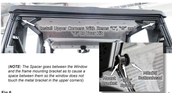
7 . After the Windshield is in place, you can now replace the long metal strip you removed earlier which goes between the window and the vehicle frame. You will use the (5) Pry Rivets, Item-"H" in your kit to attach the window to the vehicle. This will secure it to the vehicle along the bottom edge. See Fig.7 below.
