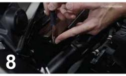
SECURELY TIGHTEN THE AMPLIFIER TO THE MOUNT
