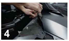
SECURELY TIGHTEN THE BUTTONHEAD SCREWS AND WASHERS TO THE TOP OF THE FIREWALL MOUNT
