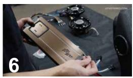
PLACE THE LONG BOLTS WITH WASHERS INTO THE AMPLIFIER MOUNTING HOLES
