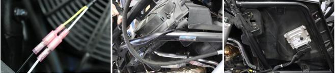
We recommend removing the Right-Side plastics to make it easier to install the harness and the Turn Switch. Run the rest of the harness with the four-pin connector along the frame through the side panel up to the Flasher Control and plug into the mating connector, make sure to keep the harness away from any hot or moving parts, secure with provided cable ties.
