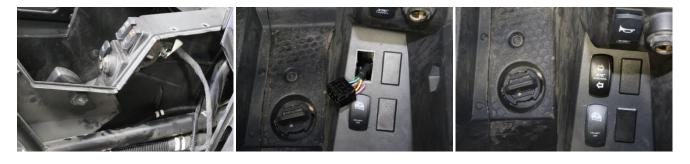
7. **Dielectric Grease** - Open the grease and put on the switch terminals and the connector terminals, the more the better, also put some on the Flasher terminals. It should also be used on any extra switches that you may have installed.
