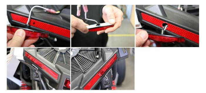
5. **Run the Rear Harness** - Start at the right rear of the car and attach the Green and White wires to the right rear LED, the Green gets attached to the black wire and the white to the white wire. Run the other Yellow and White wire to the driver's side LED the Yellow wire gets attached to the black wire and the white wire goes to the white wire. **NOTE: Black wire is positive, and the White is ground, they will not work if reversed.**
