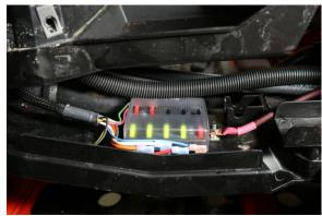
**5.** Mount the barrier strip on the dash support 1.25" bar with the provided self tapping screws. We now include our UNI-GND-RDS ground kit. Mount the ground on the bar next to the barrier strip using the supplied self tapping screws. Attach the ground wires from the items being powered to the radius ground.
