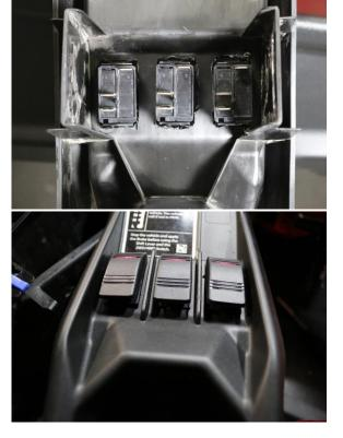
10. Run the Red 8GA power wire from the fuse block stud to the factory busbar fulltime power (Center Stud), secure the 50-amp Circuit Breaker with the supplied screws. Plug the 2 Way connector into the connector next to the fuse block and run over to the busbar and hook the Yellow wire to the bottom keyed power post and the Black to the top ground post.
