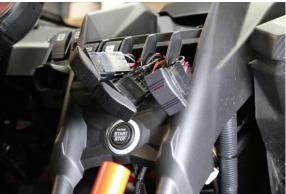
**9.** Use a cutting tool to cut out the three center console switch cutouts (Do Not Overcut, under cut and trim as needed) and mount the switches. Attach the switch harness to the switches
