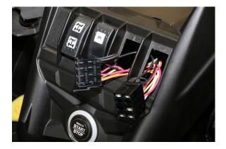
**9.** Attach the yellow wire to the switched bottom stud and the black wire to the top ground stud on the factory busbar as shown
