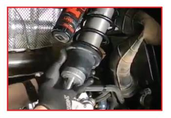
Install new main spring and OEM lower spring retainer.
