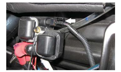
5 Unplug the stock wiring harness from the ignition coil.
