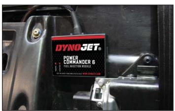
11 Plug the PC6 connectors in-line of the stock CPS and wiring harness.
