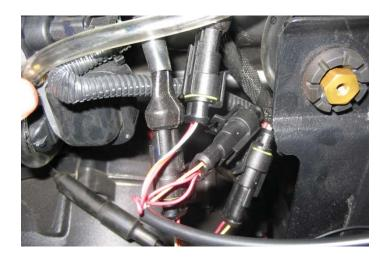
4 Connect the PC6 in-line of the stock wiring harness and the injector harness.
