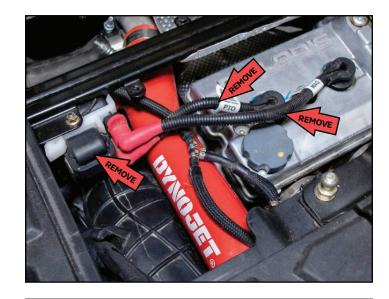
STOCK COIL AND PLUG WIRES
