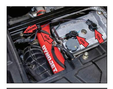
DYNOJET COILS AND WIRING HARNESS
