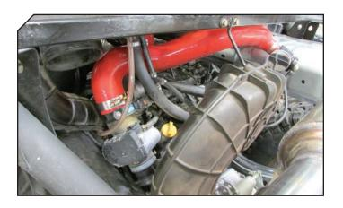
7 Install the long Dynojet boost tube on to the outlet of the intercooler and to the throttle body. Use the largest t-bolt clamp to secure the end that goes over the throttle body. Use one of the two medium sized t-bolt clamps to secure the end that goes to the outlet of the intercooler.
