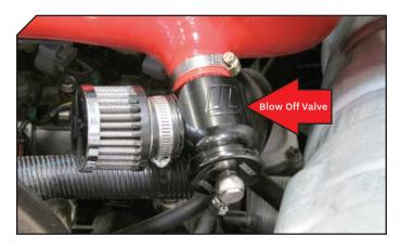
Install the blow off valve assembly into long Dynojet boost tube. Secure it with supplied hose clamp.
