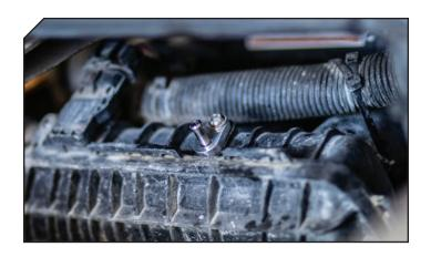
11 Install the o-ring side of the nozzle fitting into the hole of the intake plenum. Screw the plate down on top of it with the stock screw.
