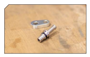
10 Replace the stock plug with the supplied nozzle fitting.
