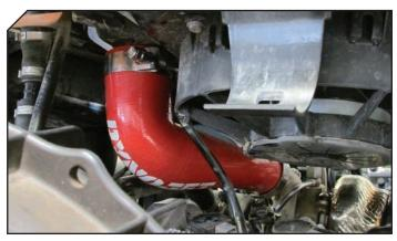
Install the short Dynojet boost tube on to the turbo and the inlet of the intercooler. Use the small t-bolt clamp to secure the end that goes over the turbo. Use one of the two medium sized t-bolt clamps to secure the end that goes over the inlet to the intercooler.
