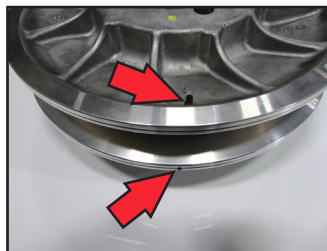
MARKINGS ON SHEAVES
