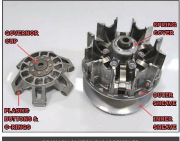
PRIMARY CLUTCH DISASSEMBLED
