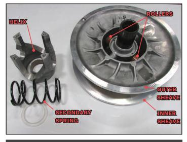
SECONDARY CLUTCH DISASSEMBLED
