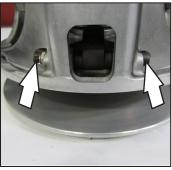
amount of weight. Refer to chart on page 2. Replace the stock spring with the Dynojet SILVER spring and reinstall the spring cover. Tighten the 6mm bolts evenly to 9 ft-lb (12 Nm).
