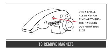
LOAD MAGNETS PER THE TABLE ABOVE. MAKE SURE EACH CLUTCH ARM IS LOADED WITH THE SAME AMOUNT OF WEIGHT.
