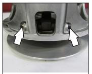
Remove the clutch arms using 3/8" socket and 1/8" allen key. Install the Dynojet clutch arms with the proper amount of weight. Refer to chart on page 2. Install the Dynojet primary spring and reinstall the spring cover. Tighten the 6mm bolts evenly to 9 ft-lb (12 Nm). Remove the secondary clutch. Use a 15mm socket to remove the retaining bolt. Remove the snap ring and slide the secondary clutch off the input shaft. Before taking
