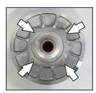
Install the supplied plastic washer to the inside of the stock spider plate.
