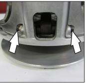
Remove the clutch arms using 3/8" socket and 1/8" allen key. Install the Dynojet clutch arms with the proper amount of weight. Refer to chart on page 2. Replace the stock spring with the Dynojet SILVER spring and reinstall the spring cover. Tighten the 6mm bolts evenly to 9 ft-lb (12 Nm).
