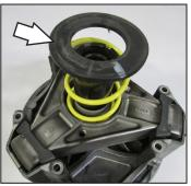
Remove the black plastic washer above the primary spring. This spacer will not be reused. Remove the clutch arms using 3/8" socket and 1/8" allen key. Install the Dynojet
