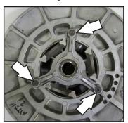
the clutch apart, be sure to mark the stationary sheave, moveable sheave, helix and cover with a reference mark. Remove the 3 torx head bolts. This cover is under extreme spring pressure. Use a clutch compression tool.
