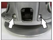
clutch arms with the proper amount of weight. Refer to chart on page 2. Install the Dynojet primary spring and reinstall the spring cover. Tighten the 6mm bolts evenly to 9 ft-lb (12 Nm).
