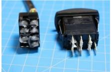
**Dielectric Grease** - Just like the OEM uses on their switches, we recommend using Dielectric Grease on all switch terminals, this keeps the water out, thereby reducing corrosion and helps increase reliability! Open the grease and put on the switch terminals and the connector terminals on both the Turn and Horn switches, the more the better.
