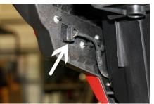
5. Drill ¾" holes in the front corners, remove the rubber grommet from the LED and insert into hole, push LED through grommet. WARNING! Verify that there is clearance before drilling holes for the LED's.
