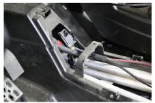
**4.** Plug rear Harness into OEM Connector - Unplug wire harness at rear left side and connect our harness, see photo below. (Note: There is a Red and Black power wire provided for an optional license plate light). Run the rest of the harness to the rear lights, Green goes to right light and Yellow goes to Left. You may leave the factory rear harness in or remove it.
